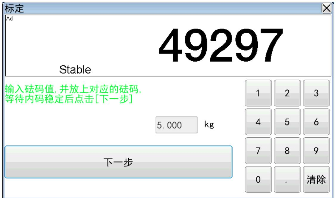
After the inside code became stable, press the next step. The calibration completed.
