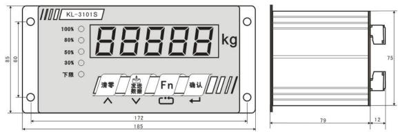
Embedded hole dimension : 151mm×76mm
