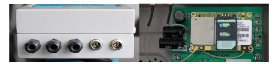
Power interface, control wire interface, load cell interface
