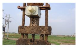
Petro pump have two main behaviour, rise and down process, both process effected on the load cell with different direction, the smallest stress probably in about  $3 \sim 5t$ , the largest in  $9 \sim 12t$  or so (different wells with different value). Waveform curve as shown below:
