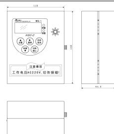
KQC-C5 instrument function is real-time monitoring and display the actual load and rated load when the load reaches its set value, the audible alarm signal, and gives the switch output. Applications: construction elevator tower crane, hanging baskets, winches, etc
