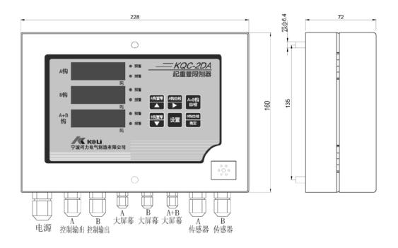
A CRANE B CRANE A+B CRANE (UNIT : TON) POWER A OUTPUT CONTROL B OUTPUT CONTROL A DISPLAY B DISPLAY A SENSOR B SENSOR
