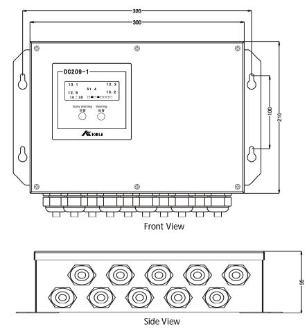
Dimension: length-300mm、width-210mm、height-95mm (not include installation part) Shell material: stainless steel Installation: wall type
